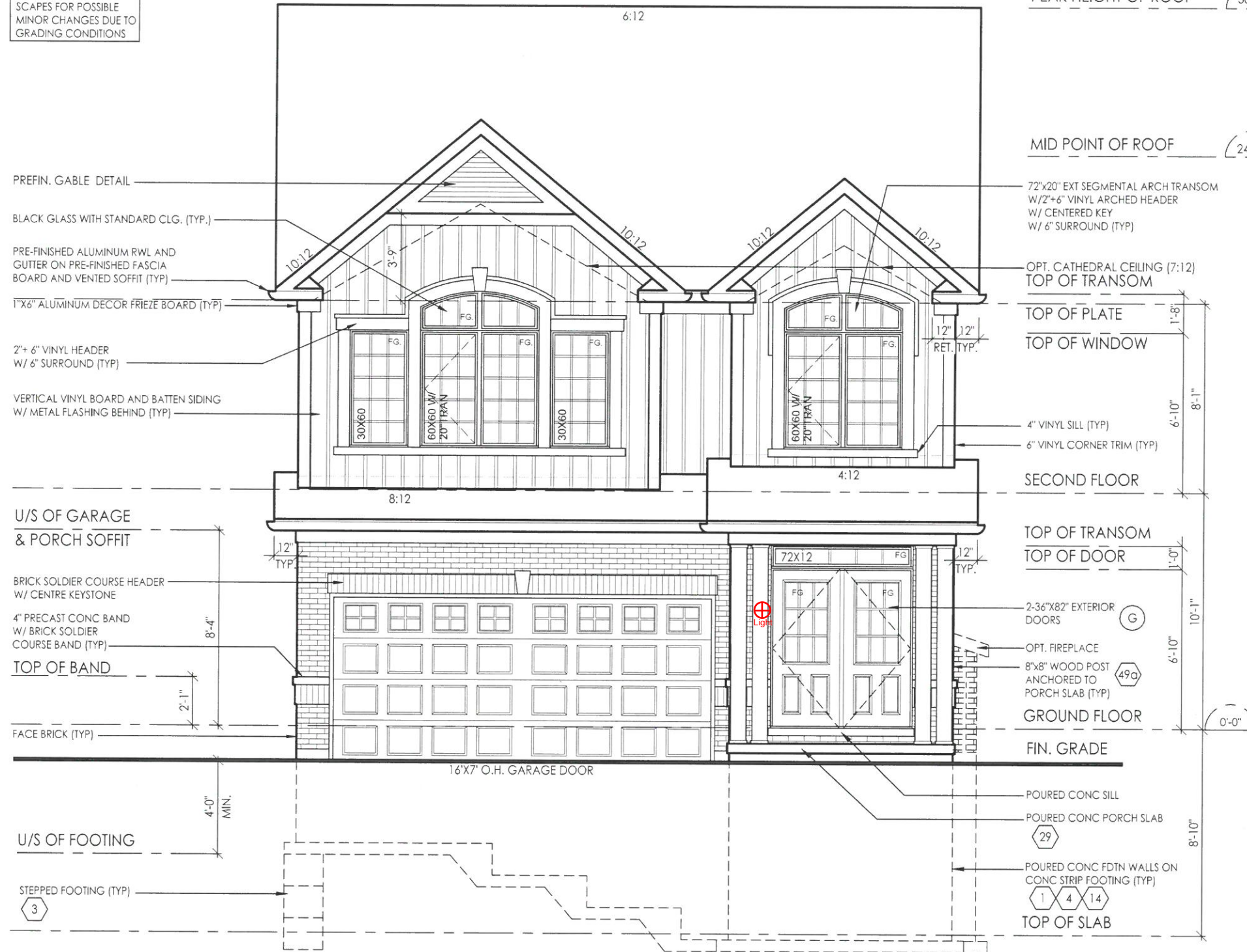
FRONT ELEVATION 'A'
